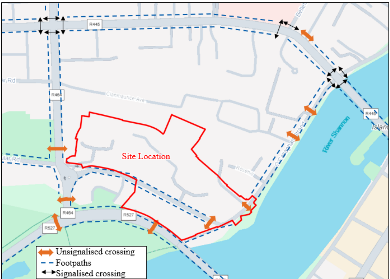
Figure 3-7 Existing pedestrian infrastructure in the vicinity of the site
