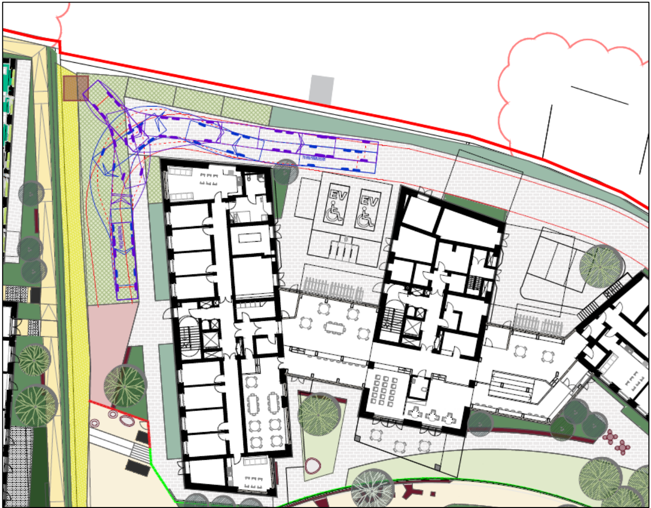
Figure 4-10 Fire tender tracking for Quarry PBSA
